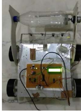
Fig.3 Final proposed prototype with LCD display
