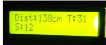
Fig.4. LCD output for the conditions of Dry soil
