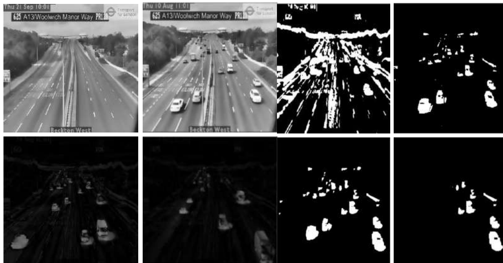
Fig.2. (a) Image of the road with no vehicles (b) After applying Bilateral Filter (c) Foreground Extraction (d) Foreground Extraction after Gaussian blur
